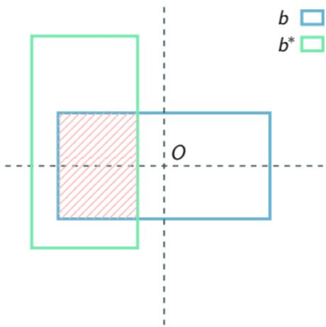
$$\begin{aligned}\text{IOU}(b^*, b) &= \text{IOU}(b, b^*) \\ &= \frac{\text{Area(red)}}{\text{Union}(b, b^*)} \\ &\leq \frac{1/2\text{Area}(b)}{\text{Area}(b)} \\ &= \frac{1}{2}.\end{aligned}$$
