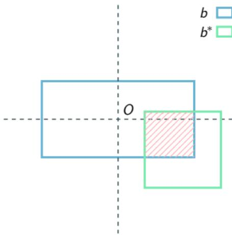
$$\begin{aligned}\text{IOU}(b^*, b) &= \text{IOU}(b, b^*) \\ &= \frac{\text{Area}(\text{red})}{\text{Union}(b, b^*)} \\ &\leq \frac{1/2\text{Area}(b)}{\text{Area}(b)} \\ &= \frac{1}{2}.\end{aligned}$$
